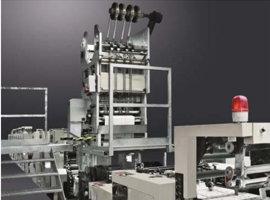
CHEETAH, a rotary hologram application system by Pantec GS Systems, installed in DongPeng, a printing company governed by Shenzhen tax department, in-line into an existing flexo printing machine.
