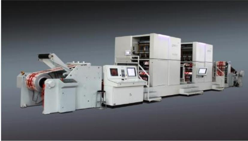
*Caption: The latest e-pack 850 refining machine equipped with two CHEETAH™ rotary hot foil stamping and patch registration systems marks the 22nd CHEETAH™ sold to the Chinese market*
