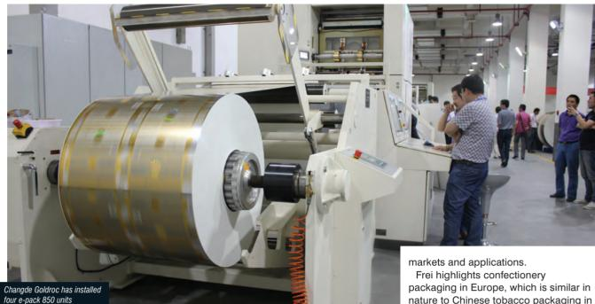
actually delivers higher overprinting accuracy than sheet-fed technology. The tolerance of a Cheetah rotary roll-to-roll machine is +/- 0.10mm.
