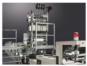
CHEETAH, a rotary hologram application system by Pantec GS Systems, installed in DongPeng, a printing company governed by Shenzhen tax department, in-line into an existing flexo printing machine.
