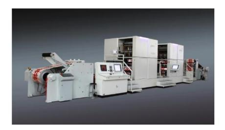
Caption: The latest e-pack 850 refining machine equipped with two CHEETAH<sup>TM</sup> rotary hot foil stamping and patch registration systems marks the 22nd CHEETAH<sup>TM</sup> sold to the Chinese market
