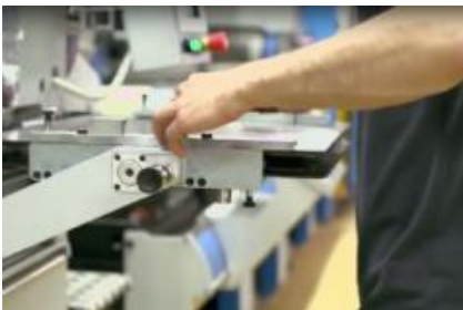
((Caption)) RHINO™ has a tool cassette for quick job change. In combination with the job saver counter plate the setup of the machine for repetitive jobs can be done without fine tuning.
